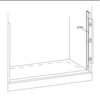
**CAUTION:** The bottom track should never be screwed to the threshold.
