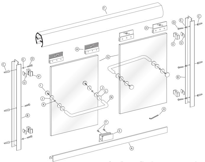
Measure the wall-to-wall opening at the center of the tub rim. Cut the tub track [A] 1/16" short of this dimension. An inexpensive miter box available at your local hardware store will help you get clean square cuts.
