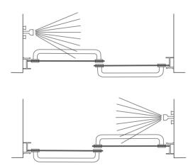
Lift the interior glass panel into position with the rollers engaging the groove in the header [F]. Repeat for the exterior panel. If panels are not parallel to their respective wall jambs, remove and adjust the rollers up or down in their slots to compensate.
